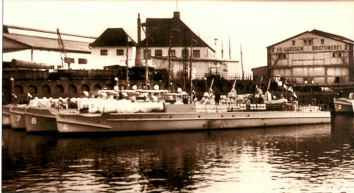
Above: The dock in front of the Lürssen factory in Bremen-Vegesack. The date is October 10, 1932 and the S6-S9 series has just finished tryouts. They will be delivered to the Reichsmarine in 1933. The dimensions of this version are slightly larger than those of the S1-S5 series. The S6 was 32.36 meters long for a 60.4-ton displacement. She was propelled by three 7-cylinder 900-hp MAN diesel engines, giving her a speed of around 30 to 32 knots. The 533-mm torpedo launching tubes and the 20-mm anti-aircraft guns at the back are still canvas-covered.
