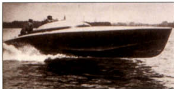
Above: The speedboat built by Otto Lürssen with which he won the world speed record in 1912. It is a small vessel, eight meters long and propelled by two Daimler Benz 102-hp engines, for a speed of more than 28 knots.
