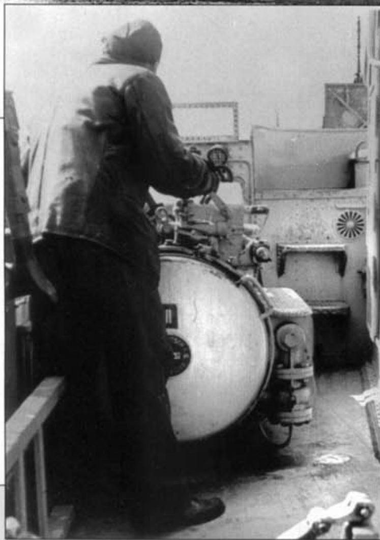
Left: The chief torpedo officer Torpedomaat has his finger on the torpedo-launching switch, waiting for the order to fire from the commander of the gunboat. After the G7a leaves the tube, the crew needs only 45 seconds to reload.
