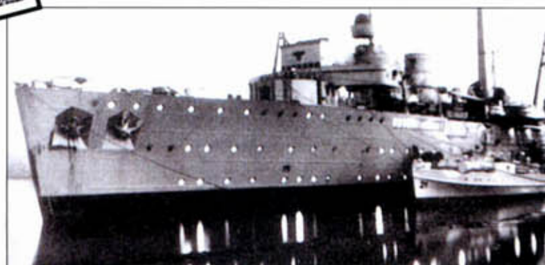
Above: The S11 training in the Baltic Sea. This snapshot, reproduced from a post card, was taken before the beginning of the war. This unit was part of the S10-S13 series, delivered in 1934. She was propelled by three 1200-hp MB 502 engines allowing her to reach a top speed of 35 knots. The S11 was turned over to the Soviet Navy in November, 1945.
