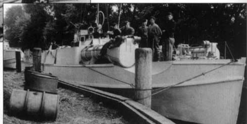
Above and right: A 3rd S-Boote flotilla transformed into an ordinary civilian vessel going through a lock on its way to the Mediterranean in October, 1941. The torpedo tube holes have been blocked and the general silhouette of the boat has been modified. All exterior weapons have been dismantled.
