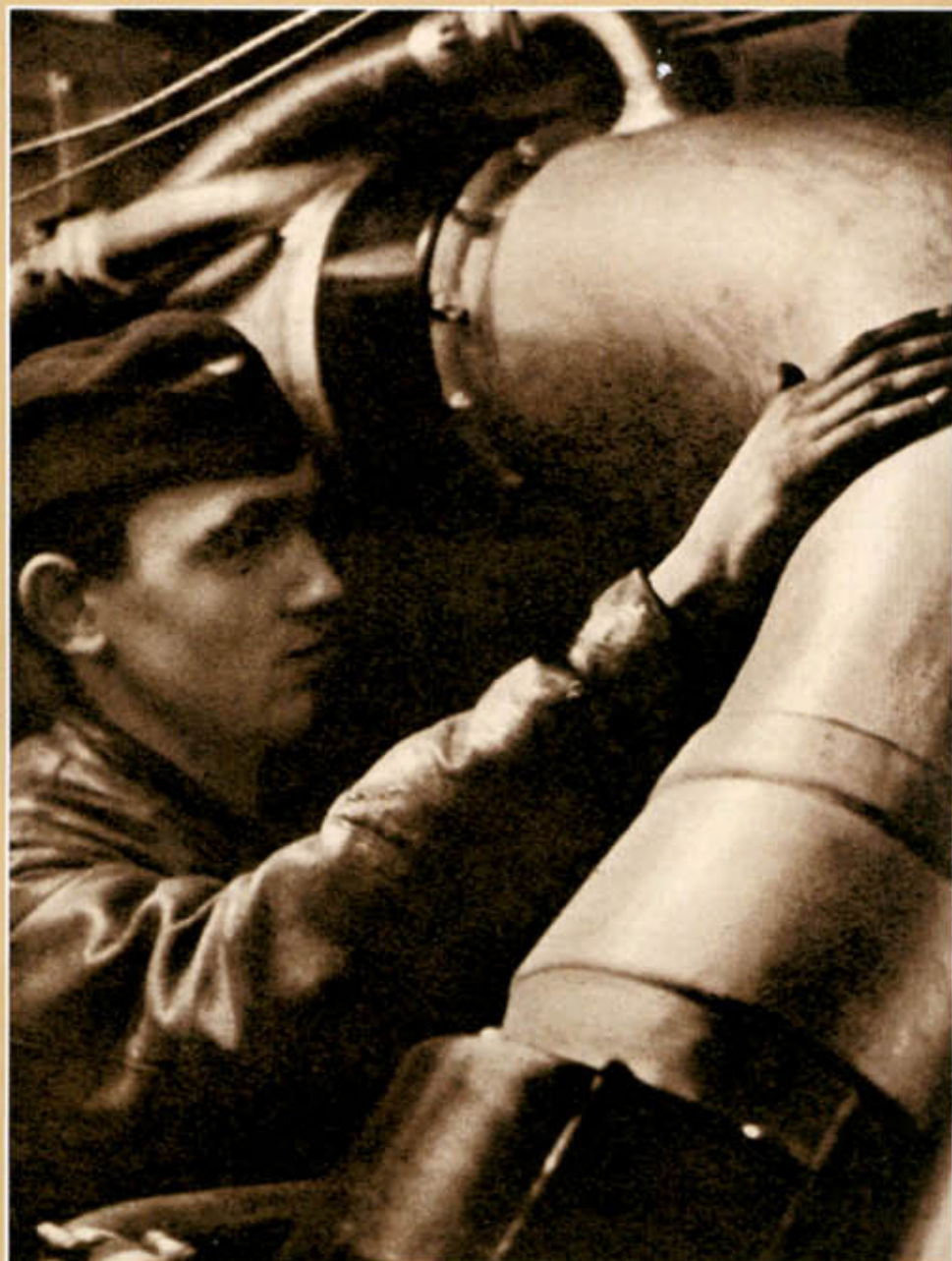
Above: Checking the temperature of the diesel engine exhaust pipes in the machine room. Half of the S-Boote crew works underneath the deck. It is difficult for these men to move around in this over-heated crowded space where they must constantly keep an eye on the three engines.
