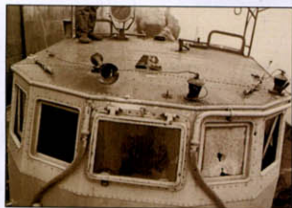
Above: Close-up view of the outside of an S-Boote bridge after a Coastal Command air raid on the port of Ostende in 1942. The structure visible here is typical of the first boats of the S38 series, not yet equipped with an armored cubicle.
