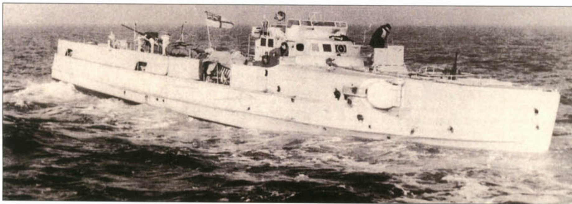
Below: The S111 after being captured by MGBs 87, 88 and 91 off the coast of Holland in the early morning of March 15, 1941. The fight with His Majesty's gunboats had been particularly violent: notice the holes made by the 20-mm guns that go right through the hull and the upper structure. The S-Boote was part of the 2nd flotilla which had attacked convoy FN 55 the night before. The British boarded the boat and took her in tow to try to get her back to England.
