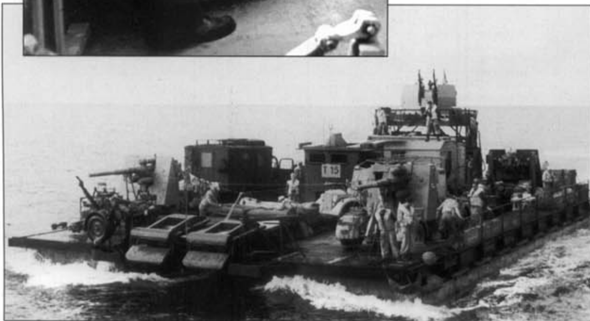
Below: A Fährprahm pictured in the Mediterranean in 1942. The ship had a large transportation capacity, and three 88-mm cannon and several vehicles are visible on board. Even though they travelled at a speed of between 10 and 12 knots, they were heavily armed. A 20-mm 4-gun Flakvierling turret was installed on the superstructure.
