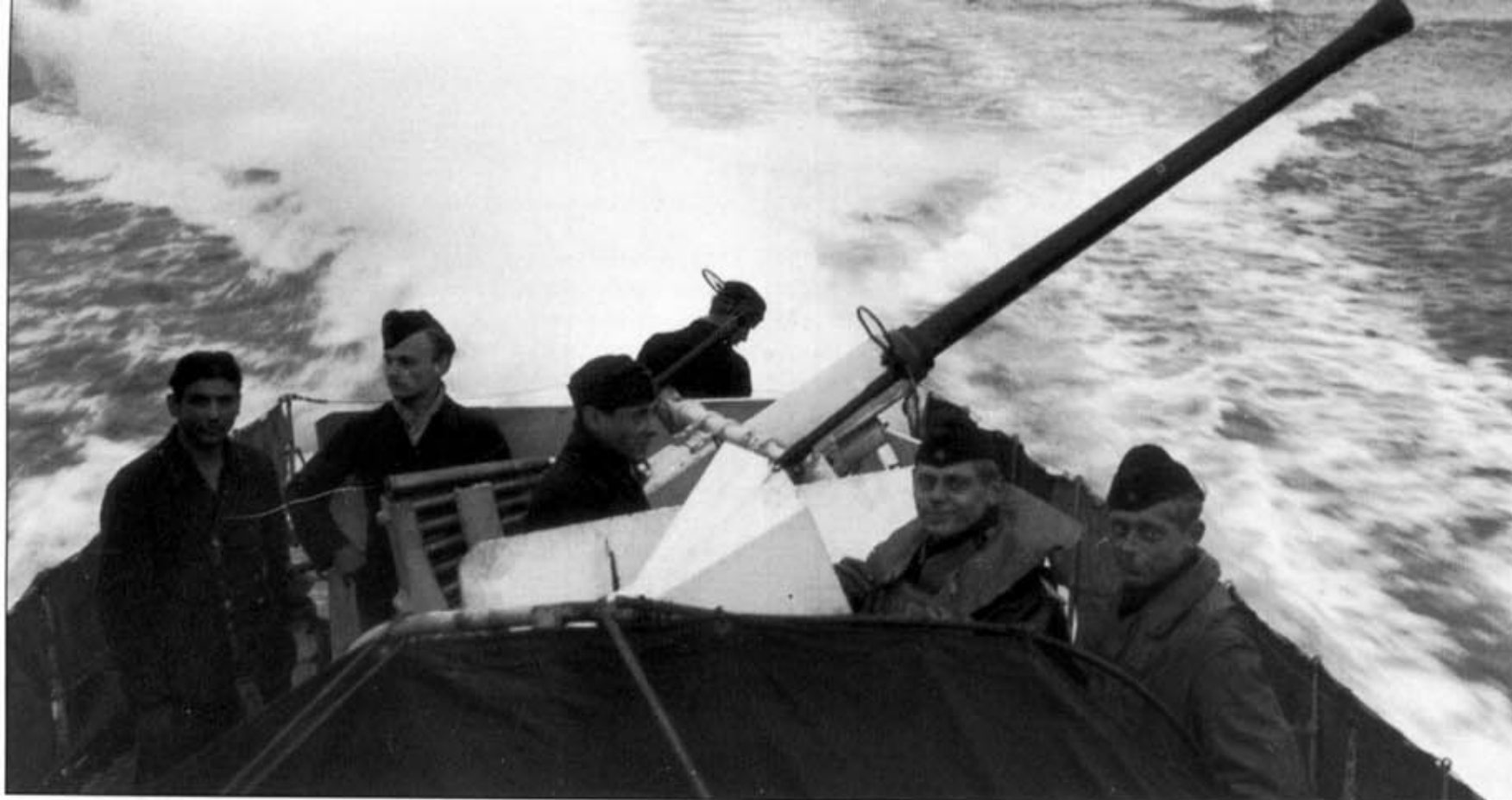
Above: A Bofors 40-mm cannon used on an S38-type S-Boote at the end of the year 1942.
