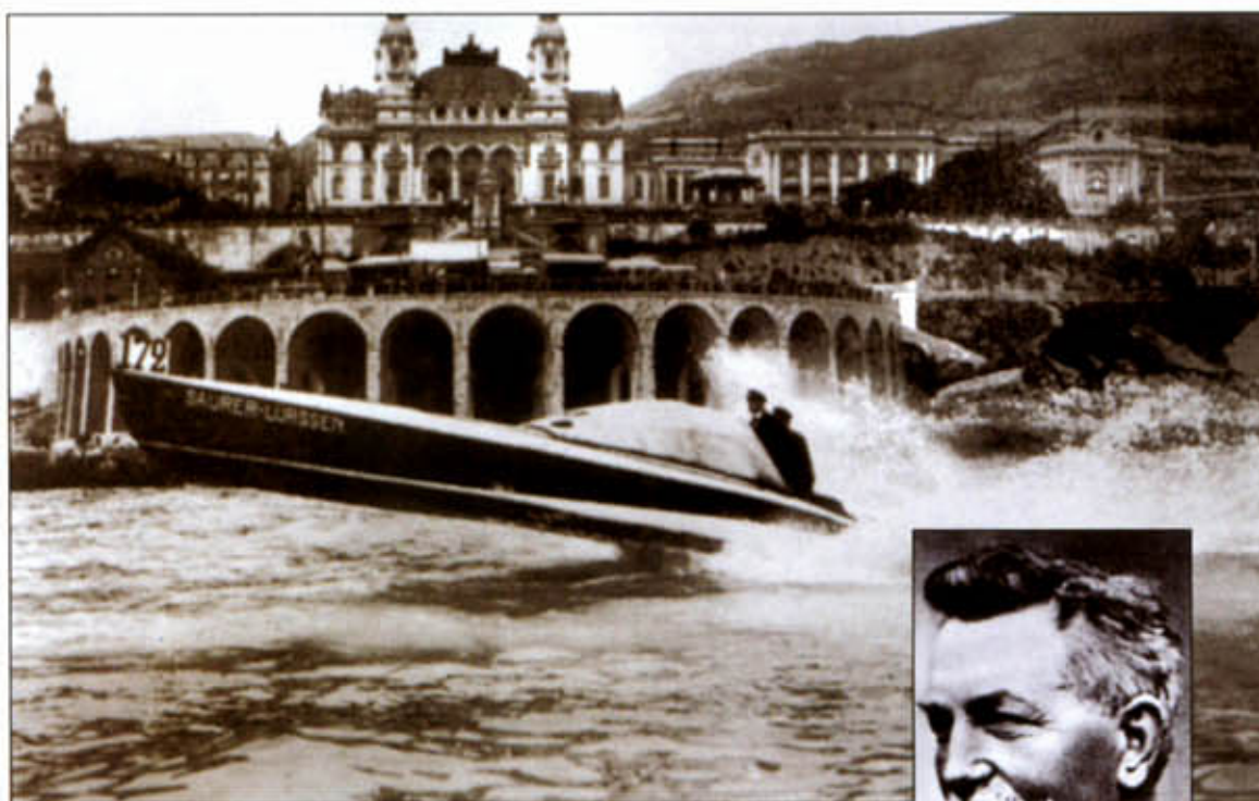
Below: The Lürssen speedboat entered in the Monaco Rally in April 1912. The boat raced in the category « 8- to 12-meter-cruisers ». The Vegesack firm had built a vessel with remarkable nautical qualities that won the event. 8,57-meters long, weighing 1712 kg, it could move at a speed of 58 km/h with perfect stability in calm or slightly choppy seas, thanks to its flat bottom and its streamlined shape.
